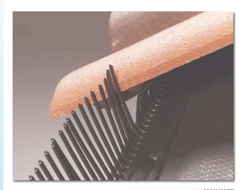
The Eaves Filler Comb is a simple and effective way of preventing birds and vermin from entering the batten cavity below profiled concrete interlocking tiles whilst allowing airflow into the batten cavity.
